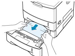
3 If you cannot find the jammed paper in the Tray2, pull the Tray1 half way out of the printer, and remove the paper.
